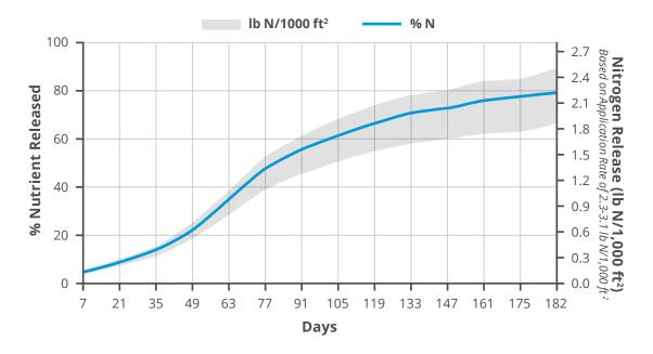
**Test Method:** Refractive index variation with dissolved fertilizer salt concentration is used to measure the percent release measurements up to 80% release.
