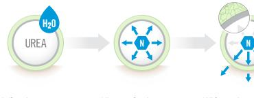
Soil moisture penetrates the sulfur and polymer coatings. Nitrogen begins to dissolve creating pressure within the granule.
